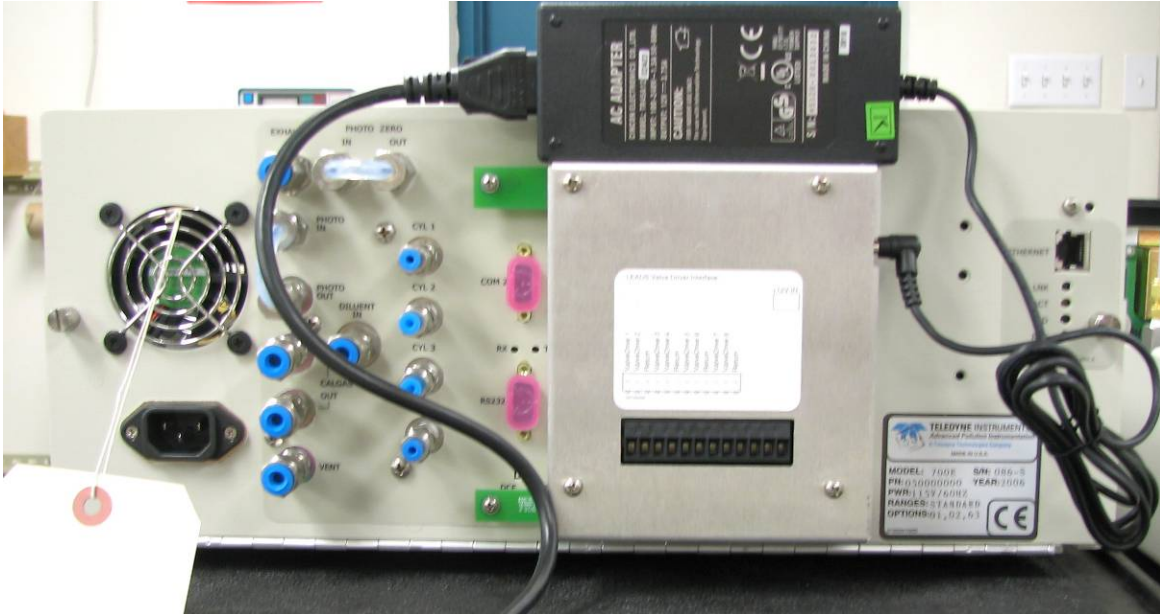
Figure 4-4: T700H Rear Panel Valve Driver Installed
