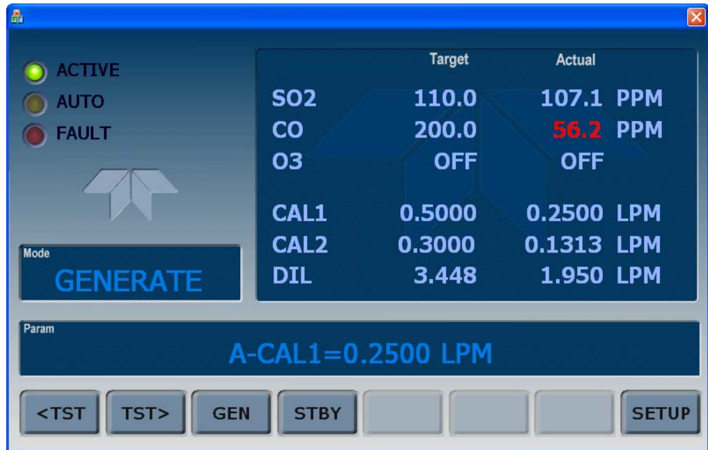
Figure 4-2: Front Panel Display when Target Values Set Outside Allowable Range
